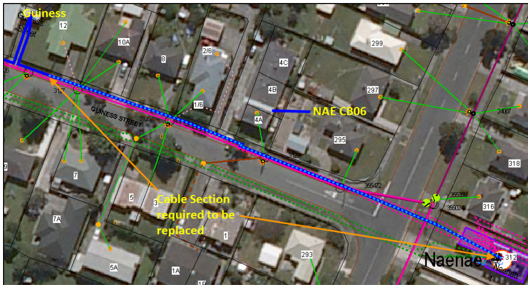
Figure 5-49 Overview of Proposed Naenae Cable Replacement
