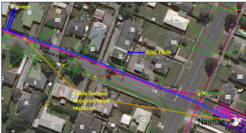
Figure 5-39 Overview of Proposed Naenae Cable Replacement
